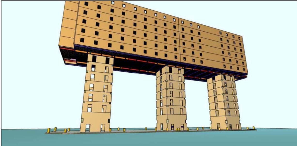
Figure 6: Rendering of visible openings in concrete cores
