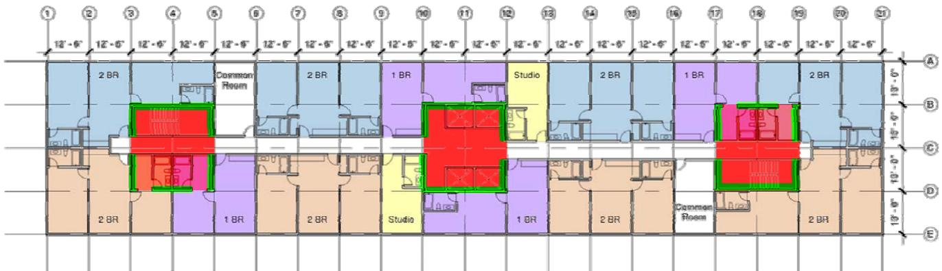
Figure 5: Typical Building Floor Plan (Core areas are highlighted in red)
